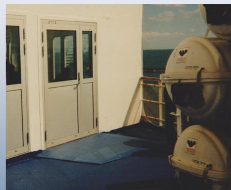
An elevated access ramp with the A-IST™ technology from SwedeSafe, onboard Stena Danica.
