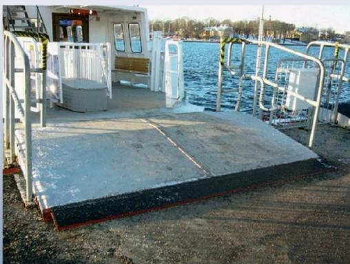
Access ramp with integrated heating function on a small passenger ferry in the Baltic sea.
